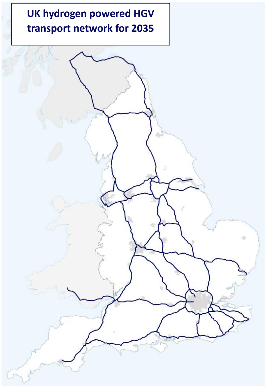
Figure 3- Map of 2035 refuelling stations network in the UK which could achieve a 50% reduction in CO 2 emissions. The network will consist of around 250 2-tonne refuelling stations. Adapted from National Highways network map. 40 Based on annual HGV flow on road network in 2016. 41
